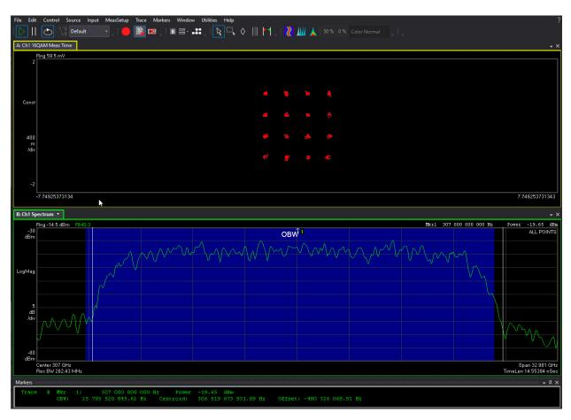
Figure 3. Conducted Measurement Results at 307 GHz for the 25.92 GHz Bandwidth Test Case
