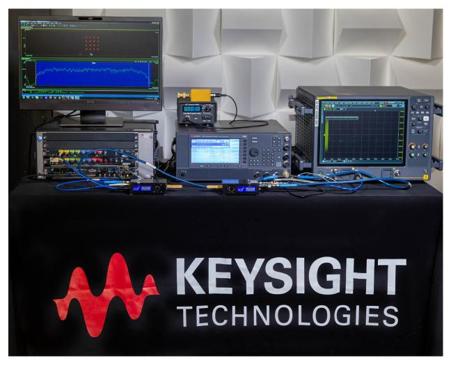
Figure 2. Sub-THz Testbed for H-Band, 220-330 GHz
