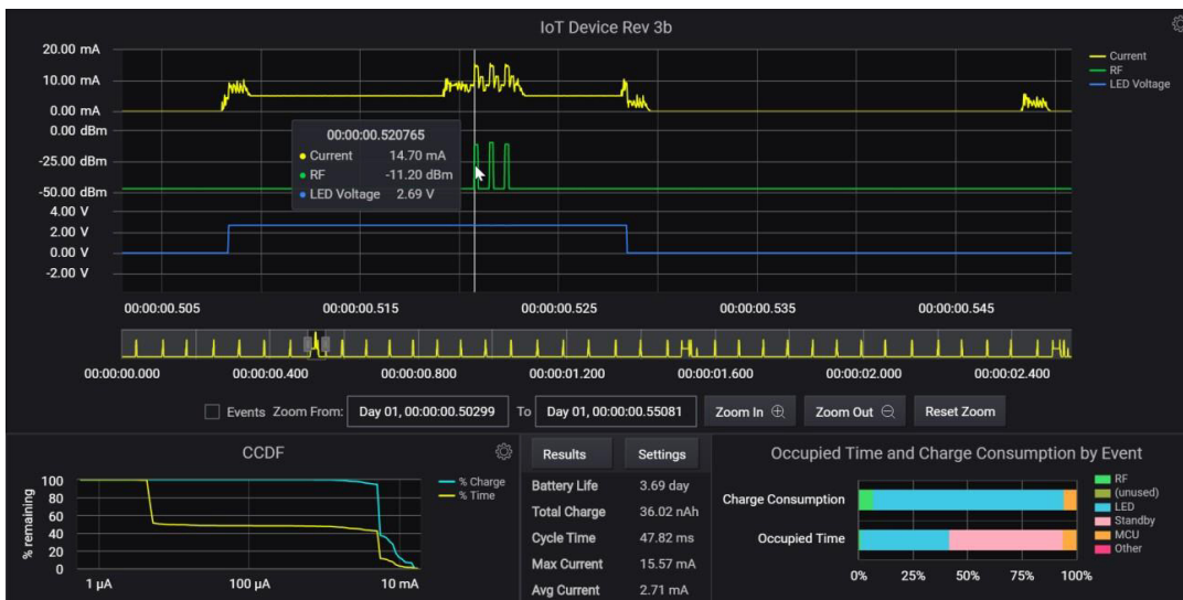
Figure 4. Event-based power analysis performed on Keysight X8712A battery life optimization solution
