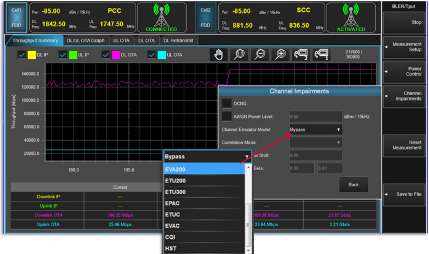
Figure 10. Reduced throughput resulting from channel impairments (fading) and recovery in throughput when the impairment is removed.
