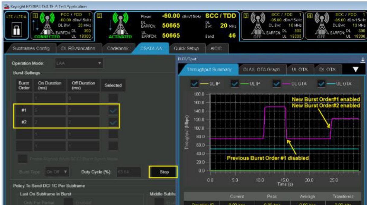
Figure 12. Base station carrying unlicensed band implements an LBT protocol to avoid collisions with a neighbor wireless system.
