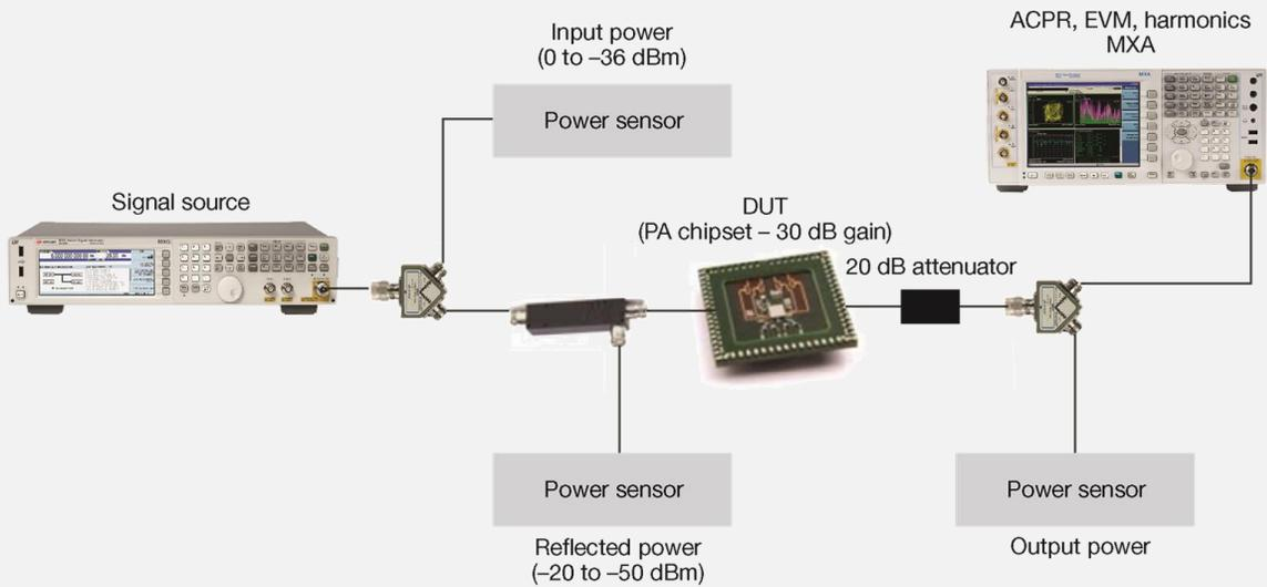
Figure 1. Typical test setup for wireless chipset manufacturing test
