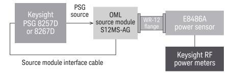
Figure 6. 60 to 90 GHz banded mm-wave source power calibration
