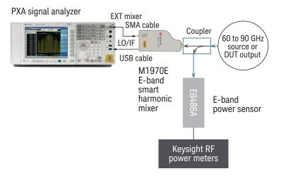
Figure 8. E-band spectrum analysis with RF power monitoring
