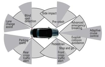
Figure 4. Overview of automotive radar functions
